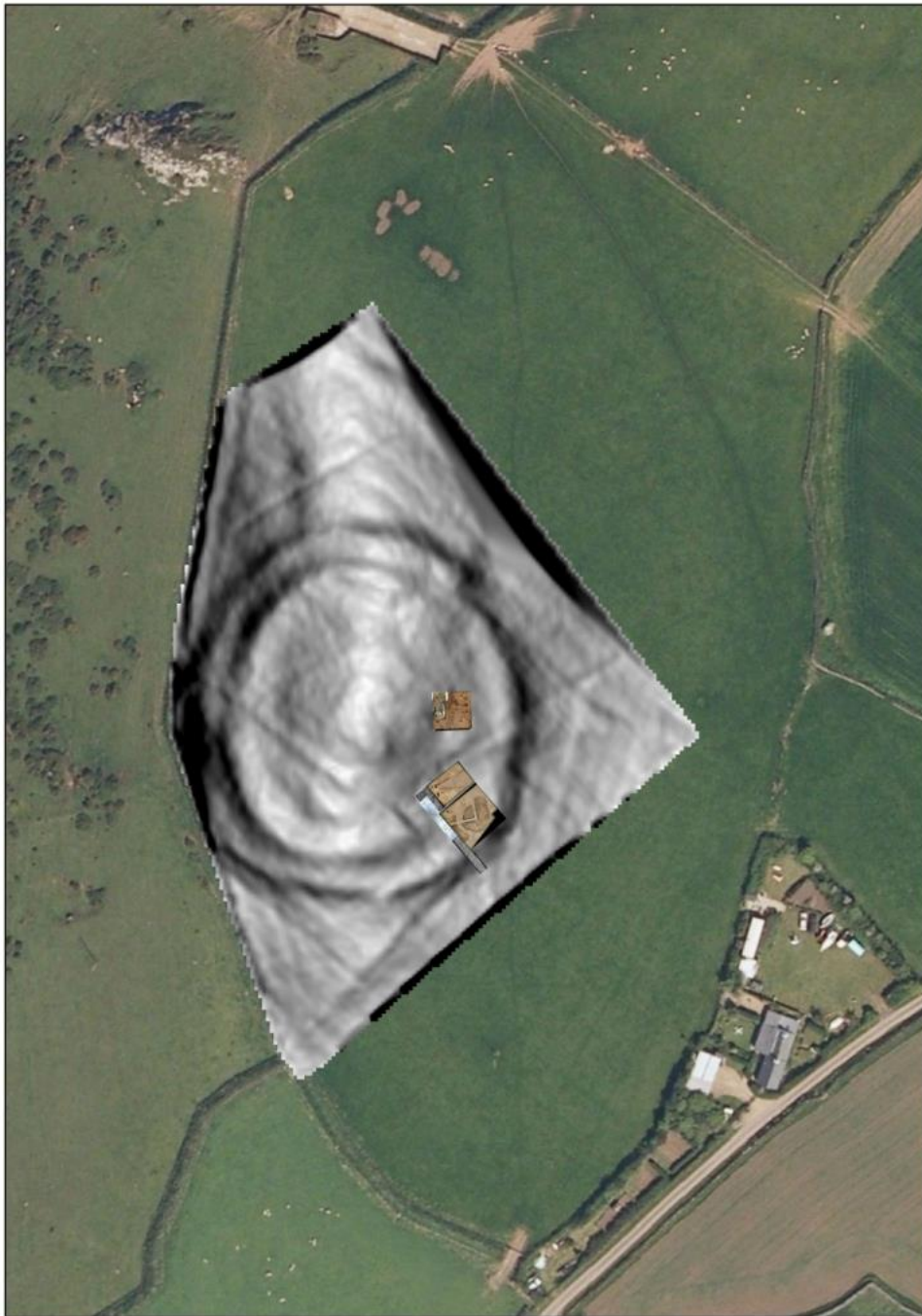
Figure 3: Digital terrain model of the site, using data from a topographic survey carried out in 2012 and presented using hillside effect. 3D photographs of the main features within each excavation area are positioned accurately over the image in Arc GIS (image: Mario Wallner). The image clearly demonstrates the slight nature of the inner bank on the eastern side of the enclosure.
